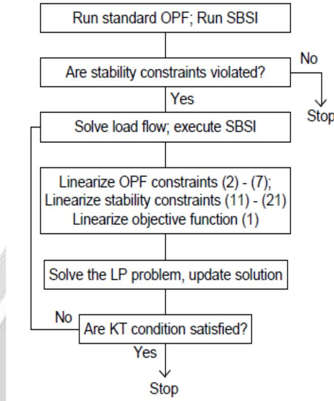
**Fig. - 1.** A procedure for the stability constrained OPF
