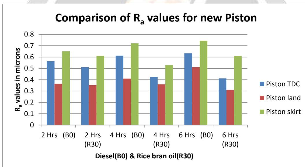
Figure 2 Comparison of  $R_a$  values for new piston (B0 and R30)
