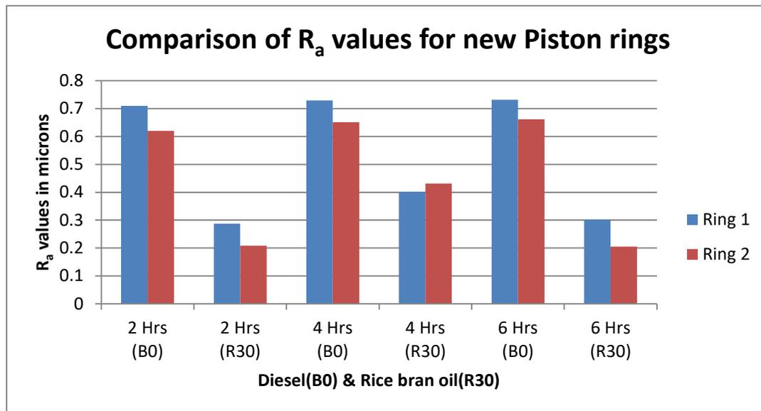
Figure 5.48 Comparison of  $R_a$  values for new piston rings (B0 and R30)
