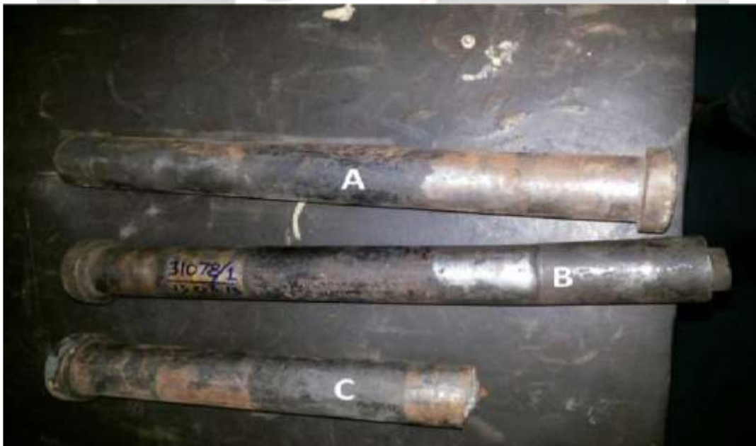
Fig.2.1 failure of knuckle pin in Mahindra 575DL
