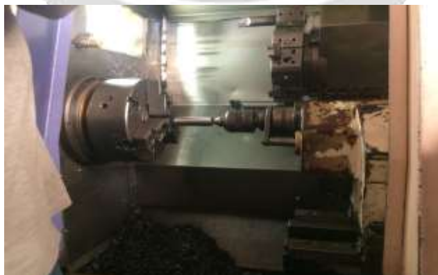
Fig. No. 3: Machining of EN36 Alloy Steel in CNC Lathe
