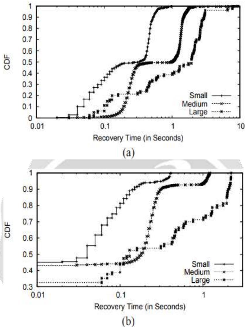
**Figure 4: Virtual network segment recomputation time underlink failures for large interactive applications on a tree topology with 30K hosts. (a) Without caching and precomputation (b) With caching and precomputation of core and aggregation devices**
