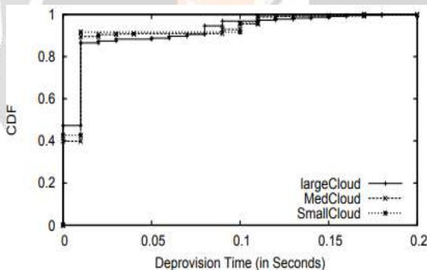
Figure 5: Virtual network deprovision time under host failures for large interactive applications on a tree topology with 30K hosts.
