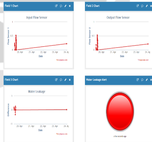
Figure14: Reading of server after leakage detection
