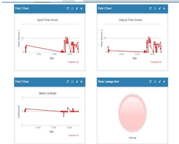
Figure13: Reading of server before leakage detection
