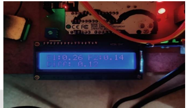
Figure11: Reading of flow sensor after water theft.
