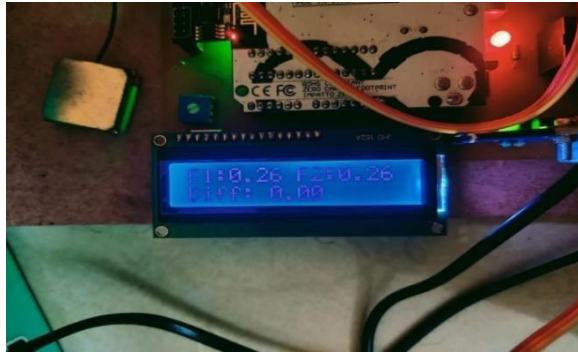
Figure10: Normal Reading of Flow Sensor
