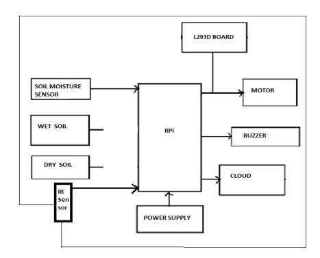
FIG - 1: Automatic Plant Watering Block Diagram
