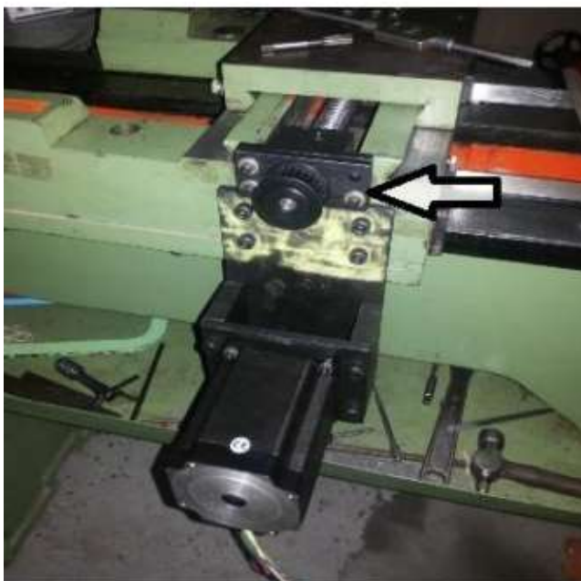
Fig. 9 X-axis mounting & stepper motor
