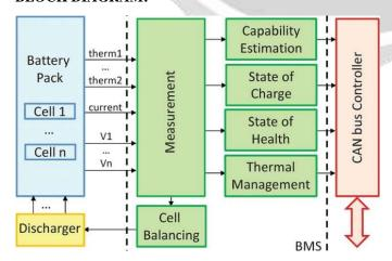
This is the diagram of battery management system (BMS), Primary functions of the BMS:
