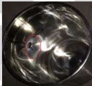
Figure 3: Steel Drum with welded anchor
