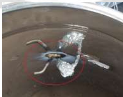
Figure 4: Anchor with strain gauge wrap with foil paper
