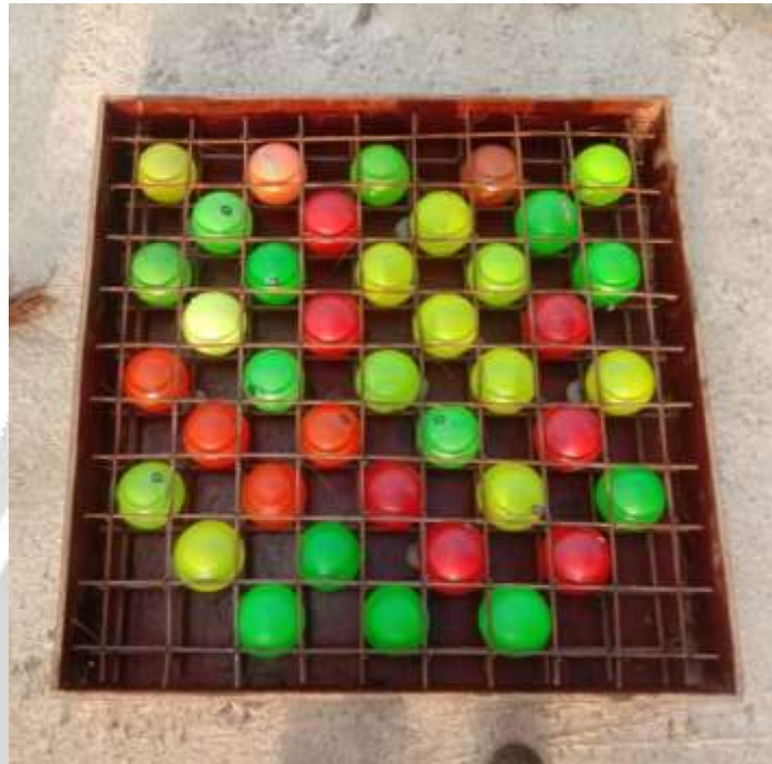
Fig.1: Bubble Deck Slab Actual Model
