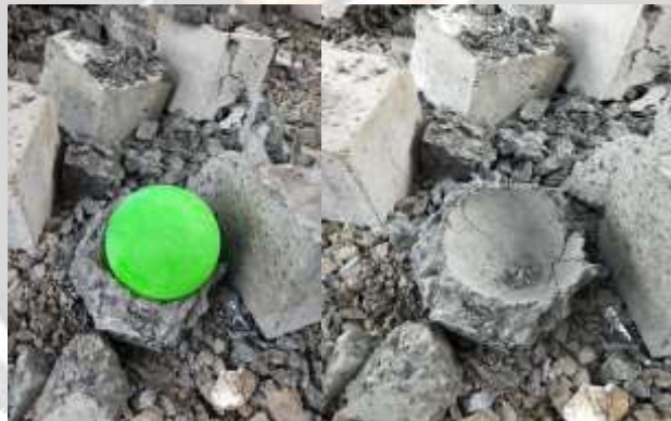
Fig.12: Ball shape forming inside of casted cube
