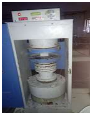
Fig-2: Compressive test of cube
