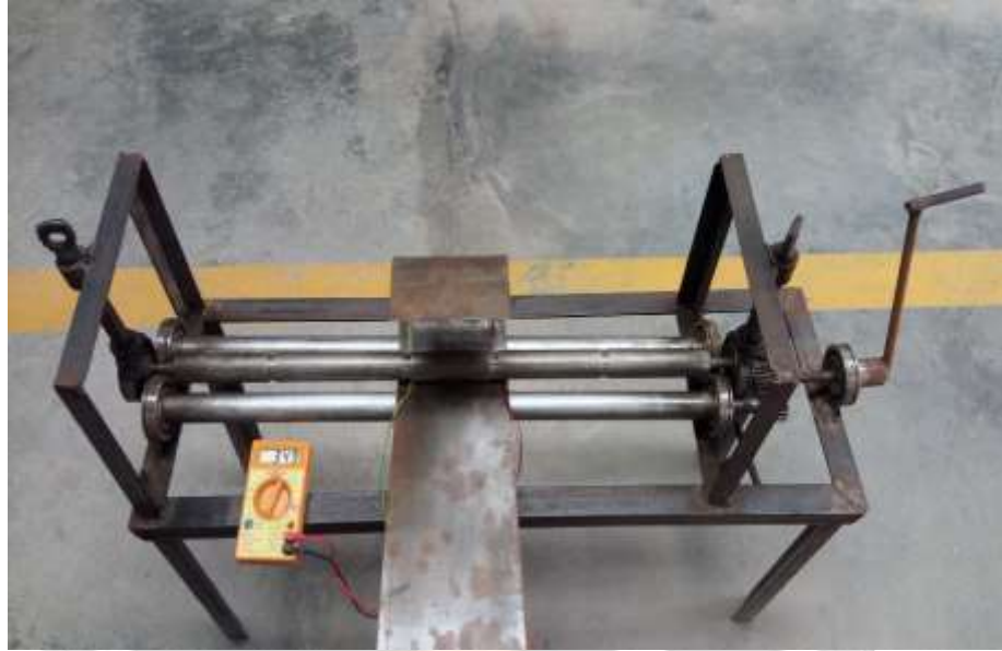
Fig.11: Experimental set up for testing on three roller bending machine.
