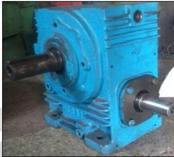
Fig.5:- Photograph of Winch Machine Gearbox
