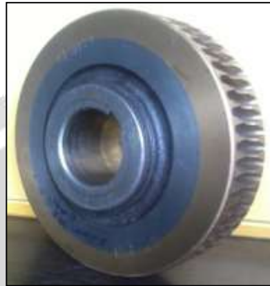
Fig.2:- Worm Wheel as a Pattern
