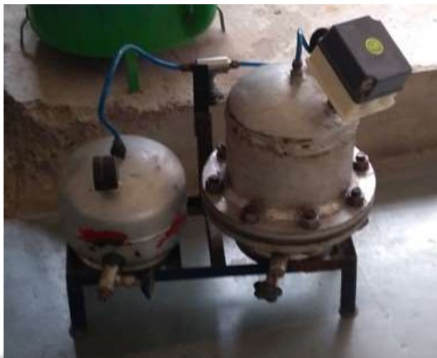
Fig. 2. One bed PSA set up
