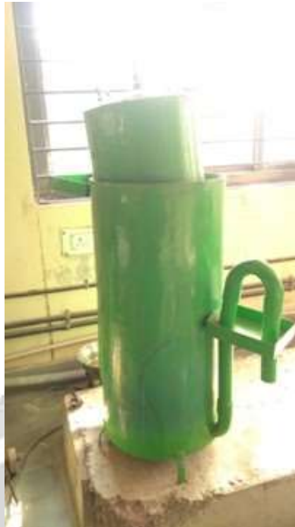
Fig. 1. biogas plant set up
