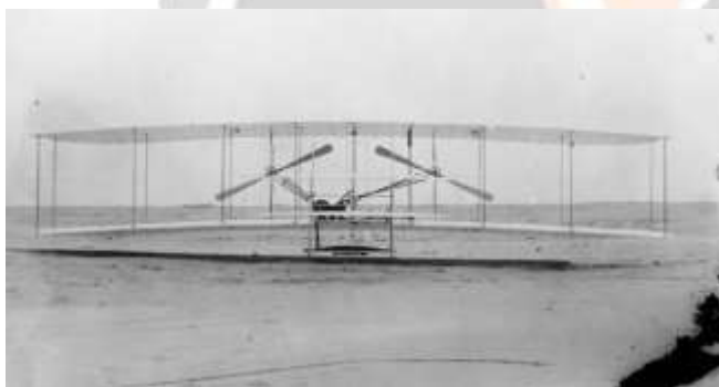
Fig-1: 1903 Wright Flyer 1 consisting of flexible wings
