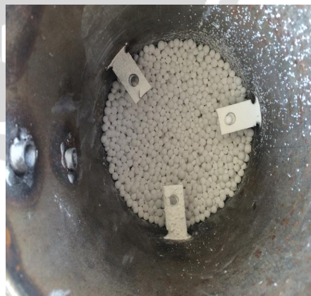
Fig-3: Catalyst and catalytic bed in reactor for CWAO process
