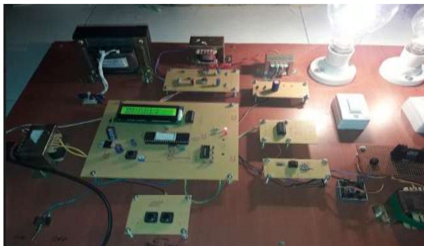
Fig-5 Hardware Snapshot of Cat Swarm Optimized Non-Superconducting Fault Current Limiter
