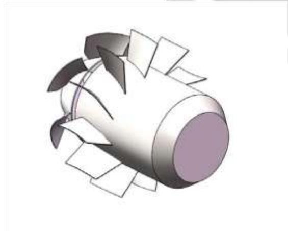
**Figure 2.** Structure of a blower guide vanes
