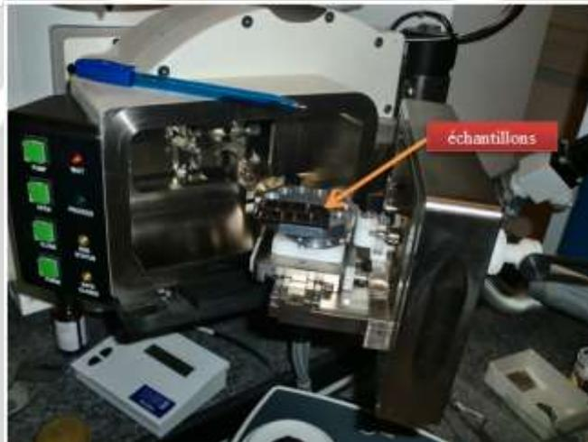
**Fig. 4: Placement of the sample in the chamber (MEB) - (Laboratoire de Géologie ENS. Lhomond .Paris V). Source: Ramanantsoa Tiandrainy. 2023**
