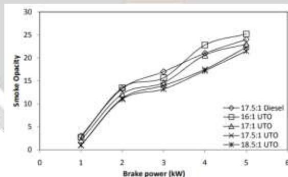
Fig. 4.30 Variation of smoke density with brake power
