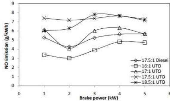
Fig. 4.14 Variation in NO emission with brake power
