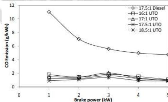
Fig. 4.11 Variation in CO emission with brake power
