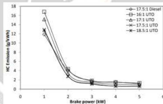
Fig. 4.28 Variation of unburnt hydrocarbon with brake power
