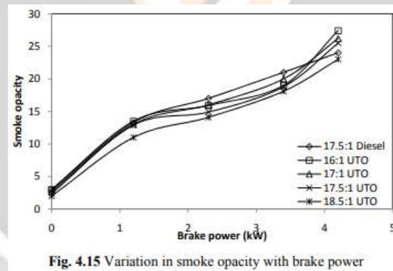
Fig. 4.15 Variation in smoke opacity with brake power
