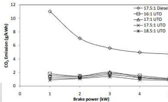
Fig. 4.12 Variation in CO<sub>2</sub> emission with respect to brake power
