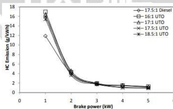
Fig. 4.13 Variation in HC emission with brake power
