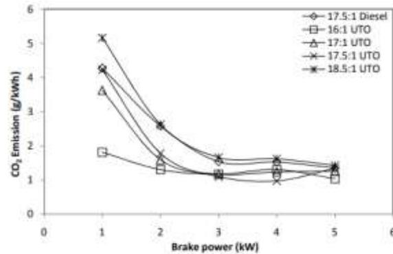
Fig. 4.27 Variation in CO<sub>2</sub> emission with respect to brake power
