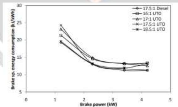
Fig. 4.24 Variation in brake specific energy consumption with brake power
