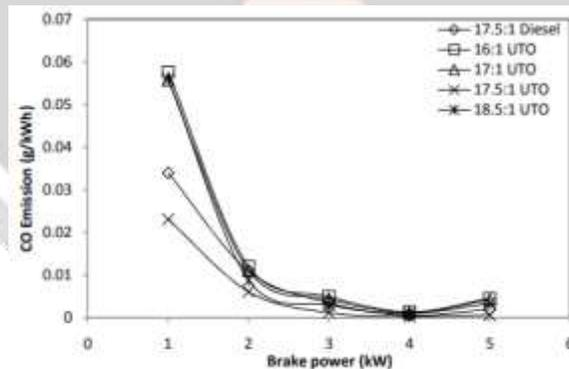
Fig. 4.26 Variation of carbon monoxide with brake power
