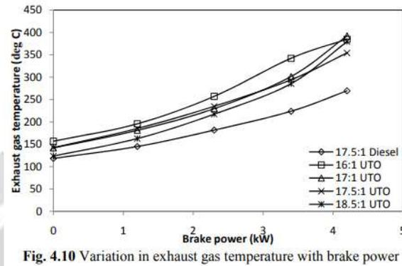
Fig. 4.10 Variation in exhaust gas temperature with brake power
