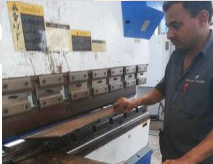
Fig 2. Cold forming of initially flat plates into Length of the beam. In innovative corrugated steel column, dimensions are same, only thickness is varie
