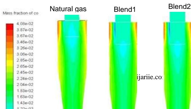
Figure 4: Profile of CO mass fraction inside the furnace obtained from 3 simulation cases
