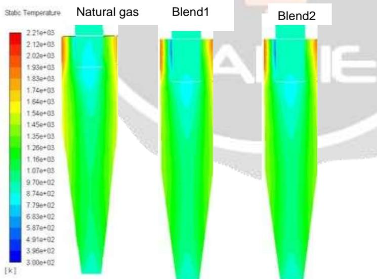
Figure 3: Temperature profiles inside the furnace obtained from 3 simulation cases
