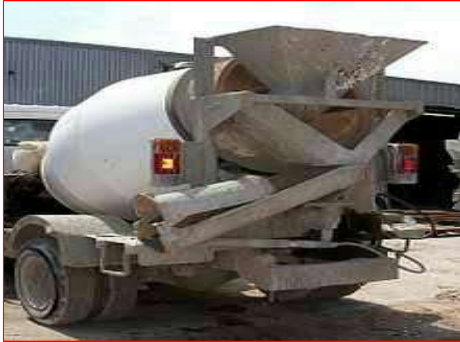
(4.1) A transit mixer carrying concrete arrangement
