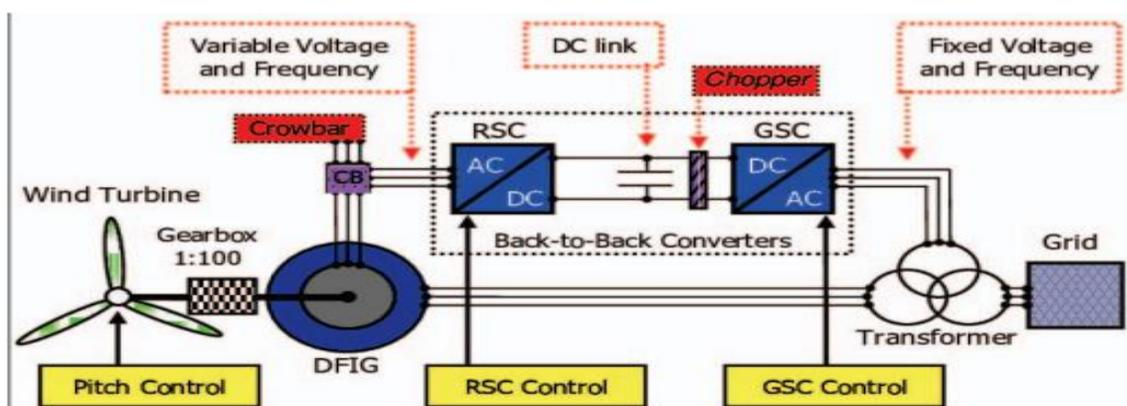
DFIGs comprise a wound rotor induction generator with its rotor circuit often regulated by power electronic devices to enable variable speed operation. The stator winding of the DFIG is directly linked to the grid via a power transformer,
