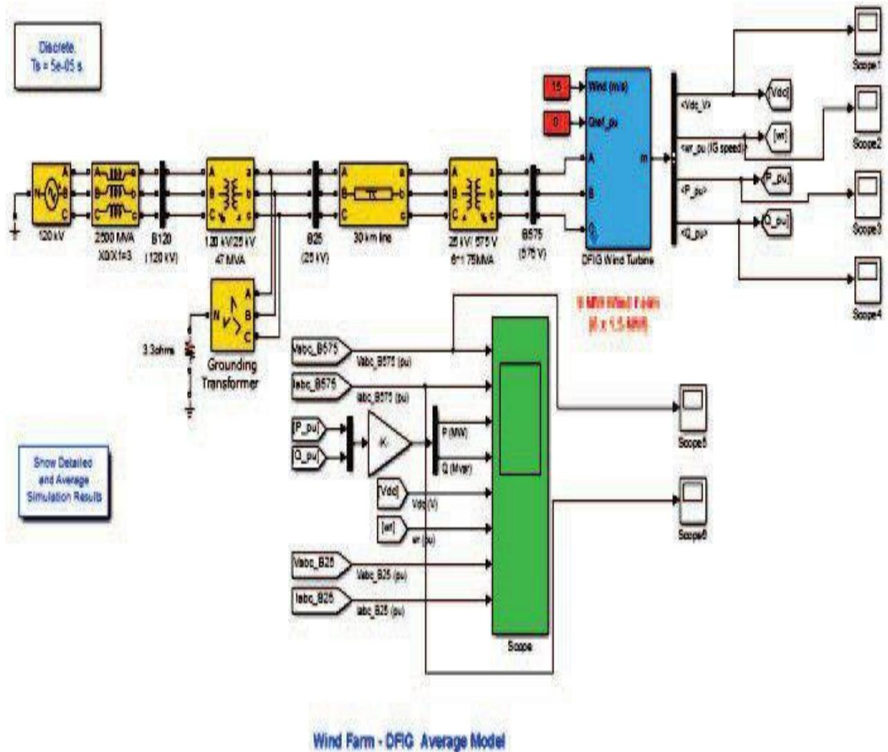
Figure 4: DFIG based wind turbine MATLAB Simulink Model diagram
