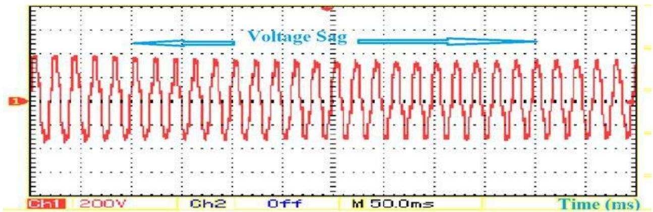
Figure 5(b): Voltages at the DFIG terminals in pu (Experimentally done)
