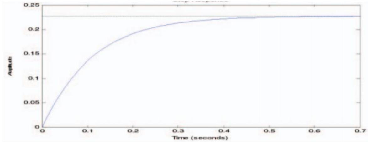
Fig 8(a) : step response of DFIG(open loop)
