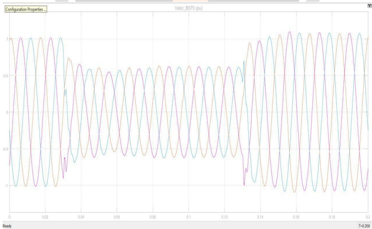
Figure 5(a) Voltage at the DFIG terminals in pu (DE-based controller)
