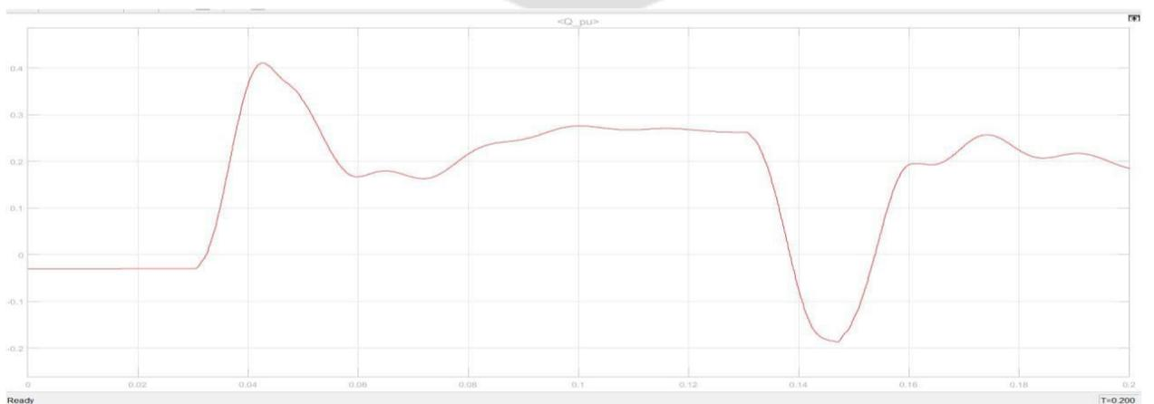
Figure 7(a): Active power requirement of DFIG in PU (DE-based controller)
