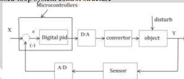
Fig -1 Structure of the control system
