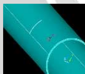
d) Radial crack (2mm)
