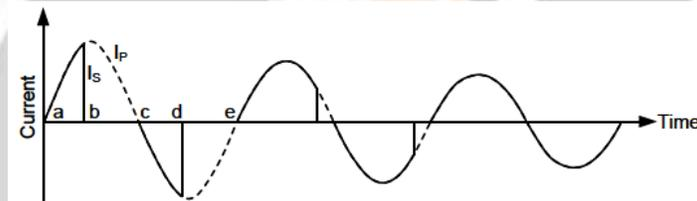
Fig -3 Primary and secondary currents, in the core during symmetrical saturation
