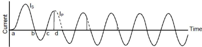
**Fig -4** Primary and secondary currents in the core during asymmetrical saturation
