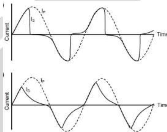
**Fig -5** Saturated waveshapes for (a) resistive and (b) resistive-inductive loads
