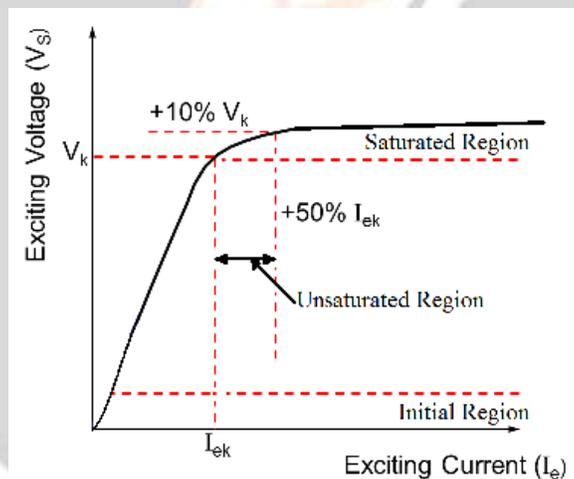
Fig -1 Secondary excitation curve representing knee-point
