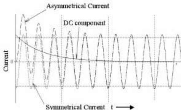
Fig -2 Fault current waveform
