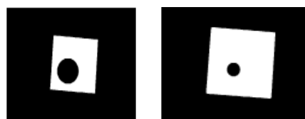
Fig 3.5.3 Morphological Erosion of a Grayscale Image
