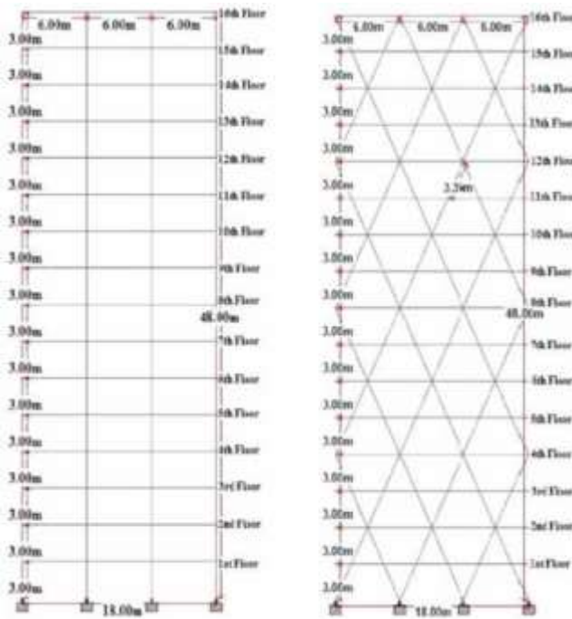
Fig – 5: Sectional view of conventional and diagrid building at 1-1
