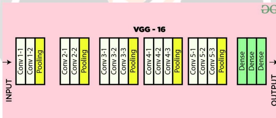
**Fig -2:** Architecture of VGG16 model
