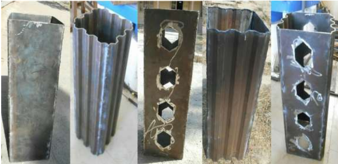
Fig 3.17 Different types of fabricated innovative HSS columns, (A) CC (B) CHSS (C) TCC (D) CCH (E) TCC
