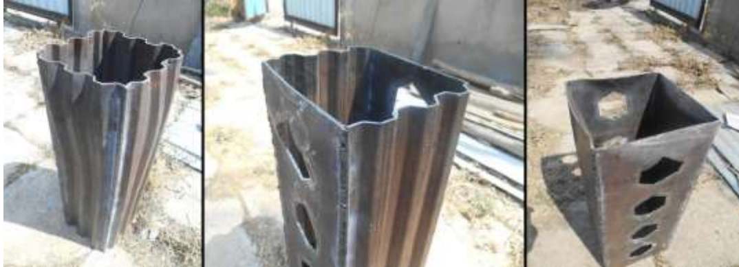
Fig 4.5 Failure mechanism for various column specimens
