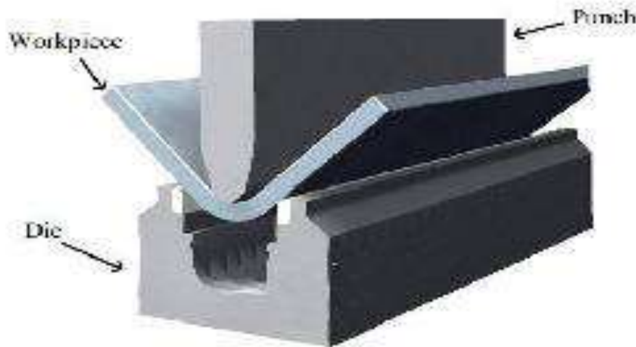
Fig 3.15 Schematic view of press-brake forming machine.
