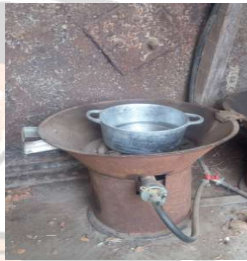
Photo 2 : Evaporation by the combustion of biogas
