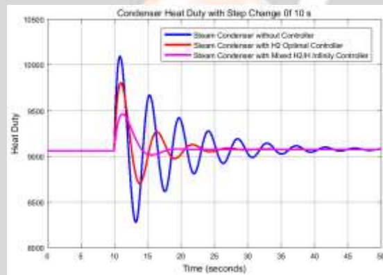
Figure 9 Condenser heat duty for a step change of 10 second
