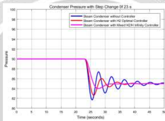
Figure 12 Condenser pressure for a step change of 23 second
