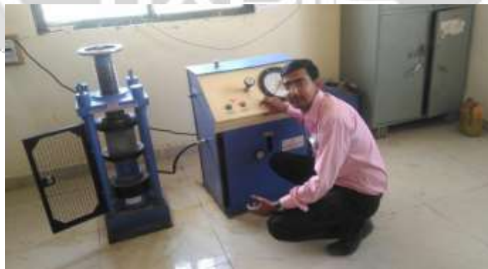
Fig.1- Compressive Testing Set up
