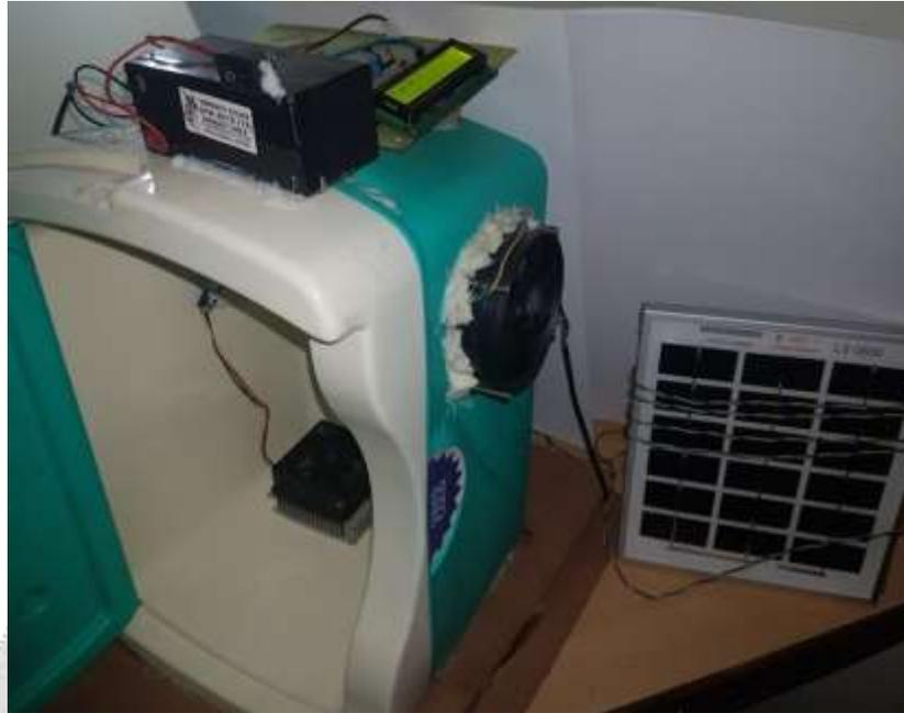
**Fig-1: Compressor Less Solar Refrigerator**
