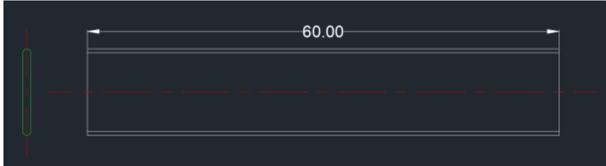
Fig – 53 Sectional view of oblong piercing punch
