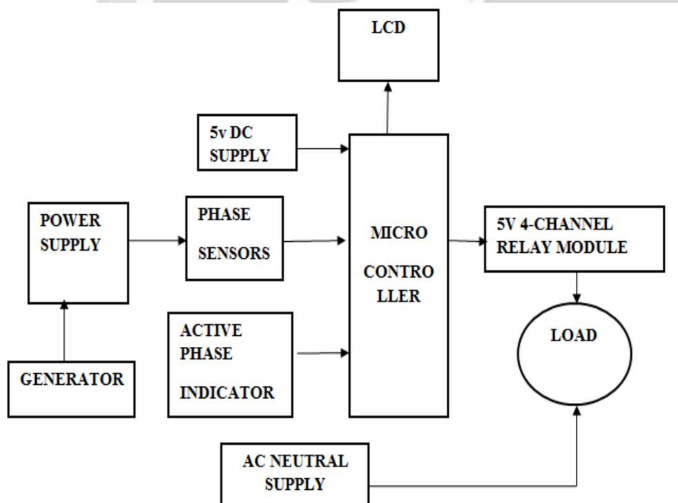
Figure1: Block diagram of Automatic Three Phase Selector
