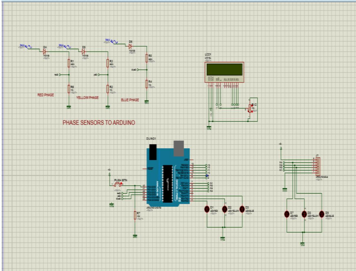
Figure 2: Circuit diagram in Proteus
