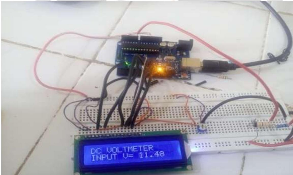
Figure 4: Connection and testing of the project on bread board.
