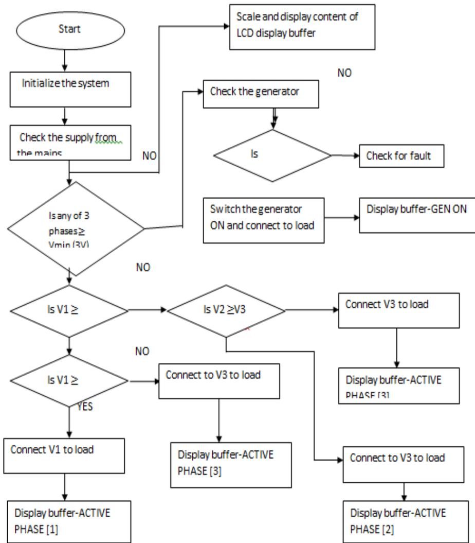
Figure 3: flow chart of automatic three phase selector
