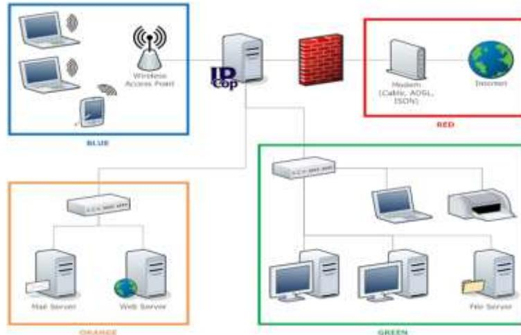
Fig -3: Four Types of Network Interfaces in IPCop
