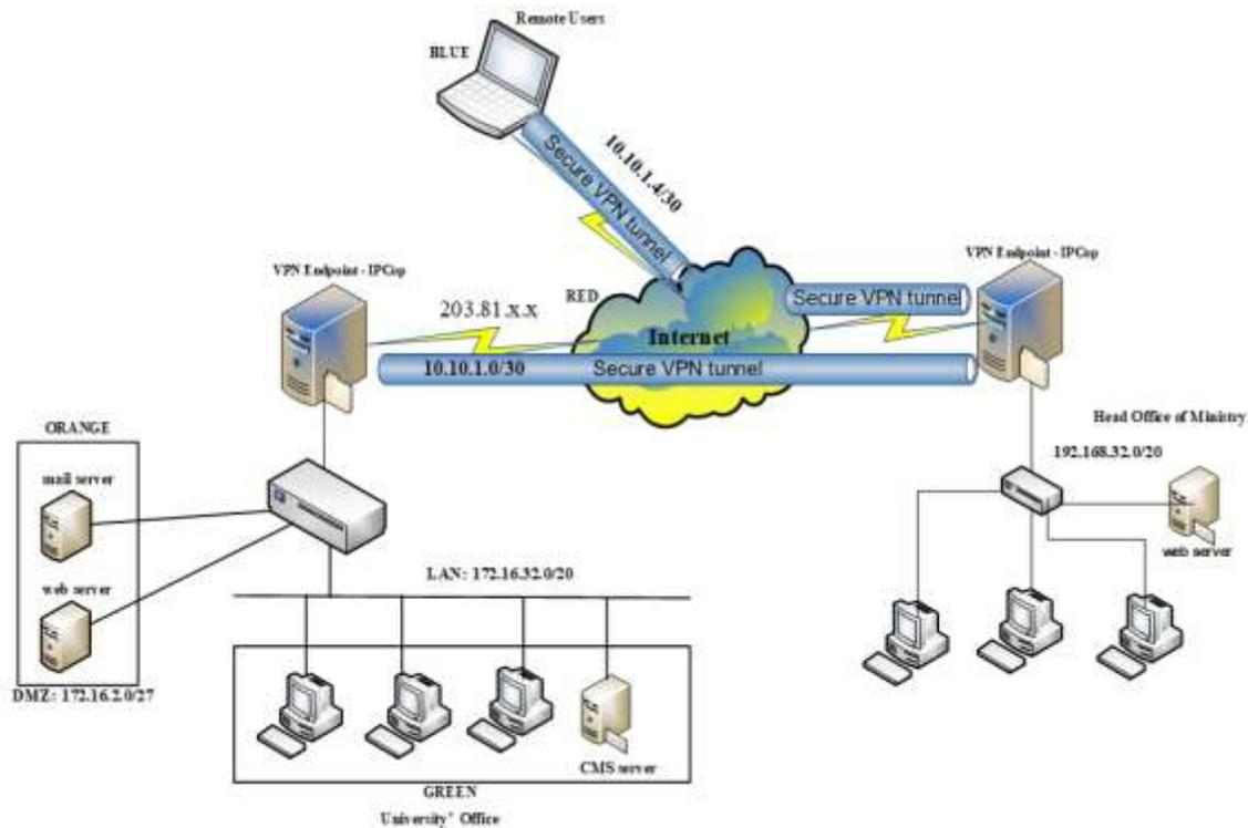
Fig - 4: Secure Connection of the University
