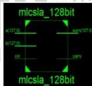
Fig-7 RTL SCHEMATIC OF MODIFIED 128- BIT LINEAR CSLA
