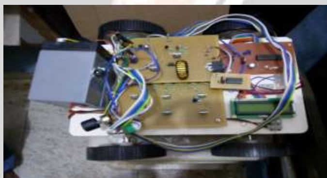
Fig 2 (b): Prototype proposed hybrid regenerative smart BLDC motor drive electric vehicle Model
