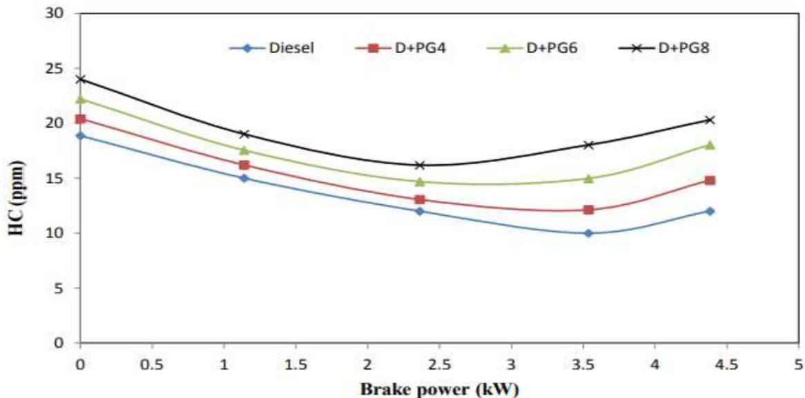
Fig. 27. Effect of brake power on HC emission at varying load in dual fuel mode
