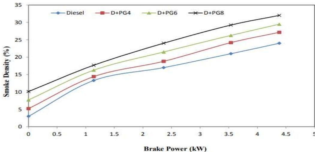
Fig. 29. Effect of brake power on smoke density at varying load in dual fuel mode
