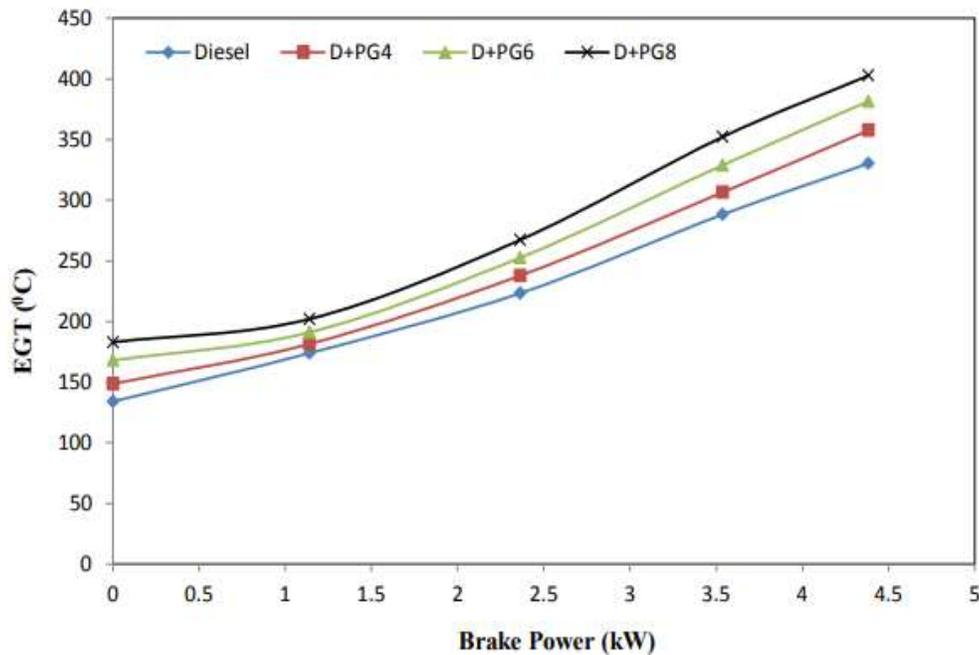
**Fig. 25. Effect of brake power on exhaust gas temperature in dual fuel mode**
