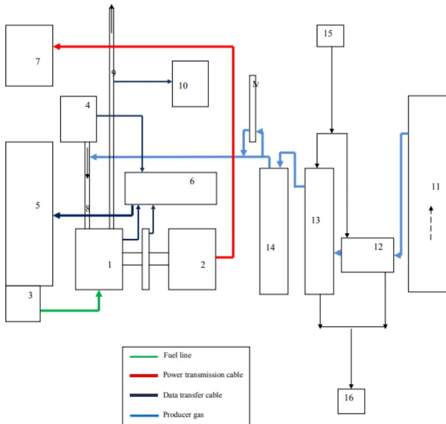
Fig. 21. Block diagram of engine coupled with gasifier
