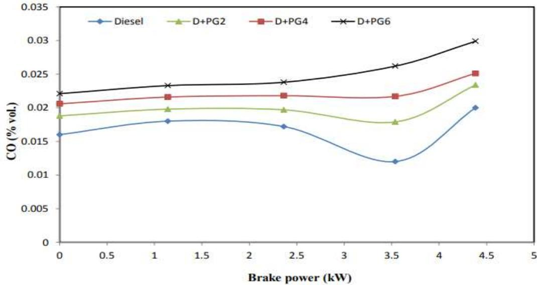
Fig. 26. Effect of brake power on CO emission at varying load in dual fuel mode
