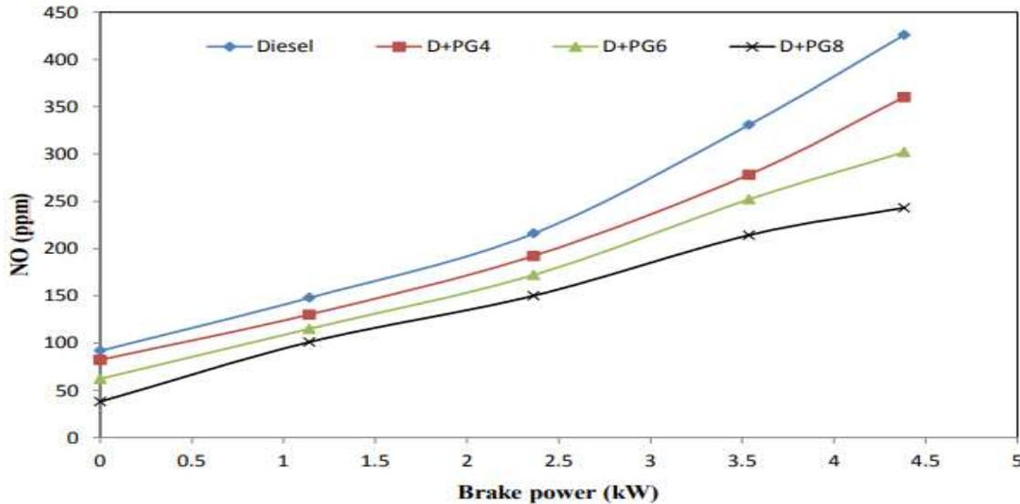
Fig. 28. Effect of brake power on NO emission at varying load in dual fuel mode
