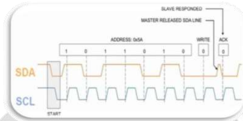
Fig-3: Acknowledge Report of I 2 C protocol
