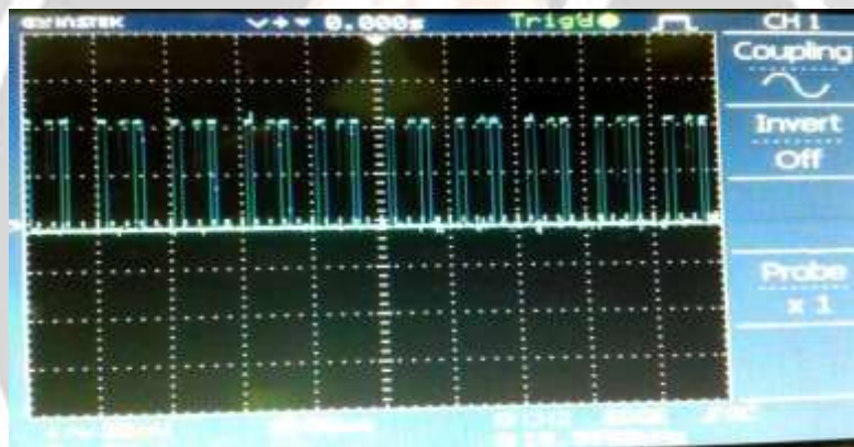
Fig 5: Wave shape of duty cycle in Boost mode
