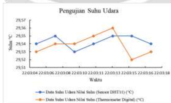
Figure-9 Comparison graph of the temperature value read by the sensor with a standard thermometer
