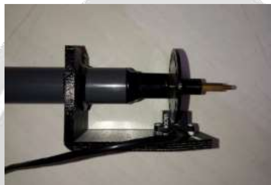
Figure-1 Optocoupler sensor construction using a rotary disk encoder
