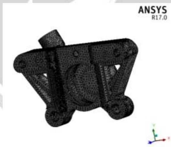
Figure 5 Meshed Model of one caliper body in ANSYS 17.0
