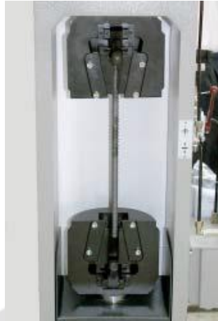
Figure 5: Detail of frame 70-C0019 with Grip holders mounted and sample inserted [6]
