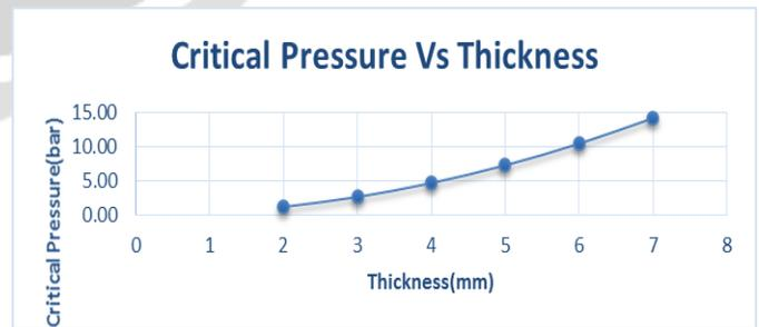
**Fig. 7** Critical Pressure Vs Thickness of Outer vessel Head
