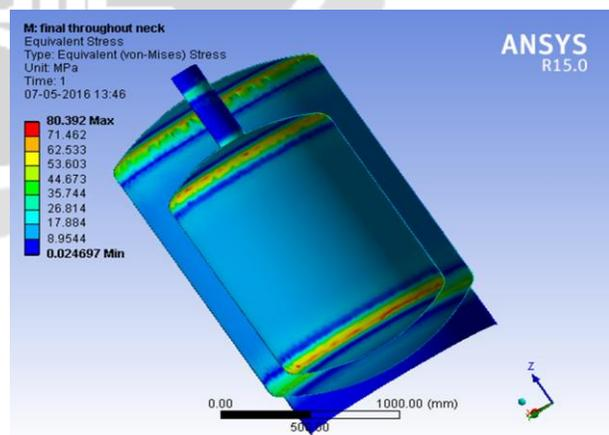
Fig. 15 Equivalent (Von-Mises) Stress in Dewar
