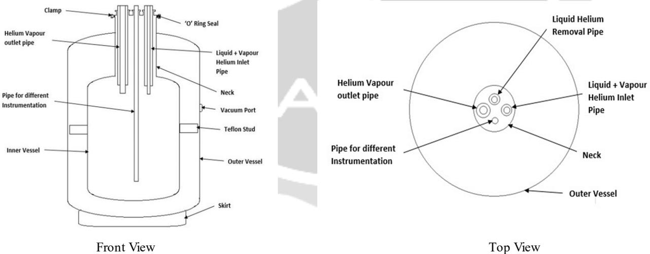
**Fig.12** Assembly of different parts of Dewar
