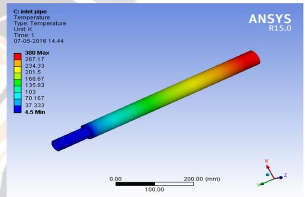
Fig. 20 Temperature Distribution in Liquid Helium Inlet Pipe
