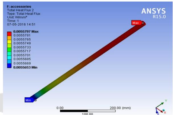
Fig.25 Heat Flux Distribution in Instrumentation Pipe
