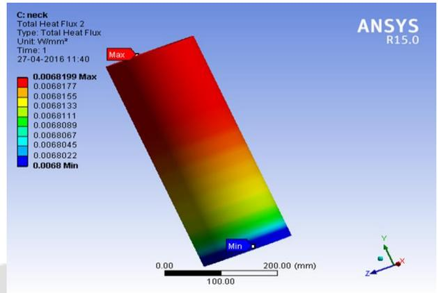
Fig.19 Heat Flux Distribution in Neck
