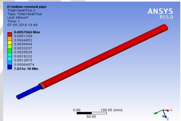
Fig. 23 Heat Flux Distribution in Liquid Helium Removal Pipe
