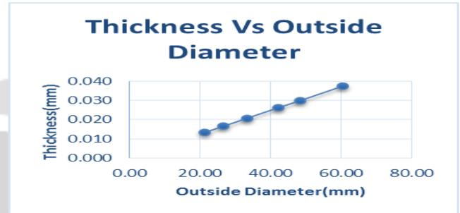
Fig. 8 Required Thickness Vs outside Diameter of Pipe subjected internal Pressure
