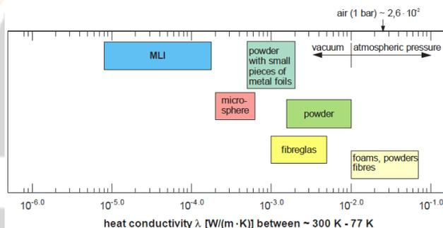
**Figure 2.** Range of heat conductivity of various insulation materials at different temperature. [12]
