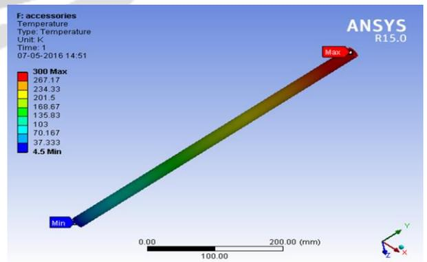
Fig. 24 Temperature Distribution in Instrumentation Pipe
