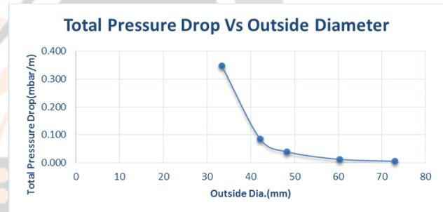
Fig. 9 Total Pressure Drop Vs outside Diameter of Inlet Pipe
