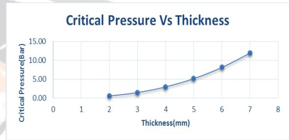
**Fig. 6** Critical Pressure Vs Thickness of outer vessel
