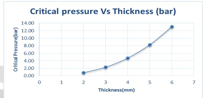
Fig. 4 Critical Pressure Vs thickness for inner vessel cylinder
