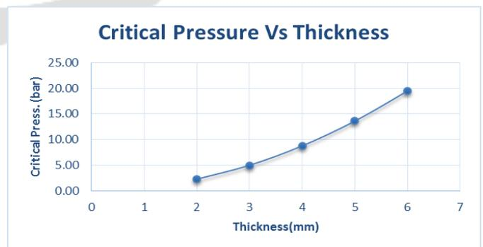
Fig. 5 Critical Pressure Vs thickness for inner vessel Head
