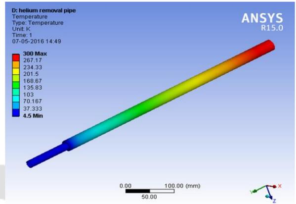
Fig. 22 Temperature Distribution in Liquid Helium Removal Pipe
