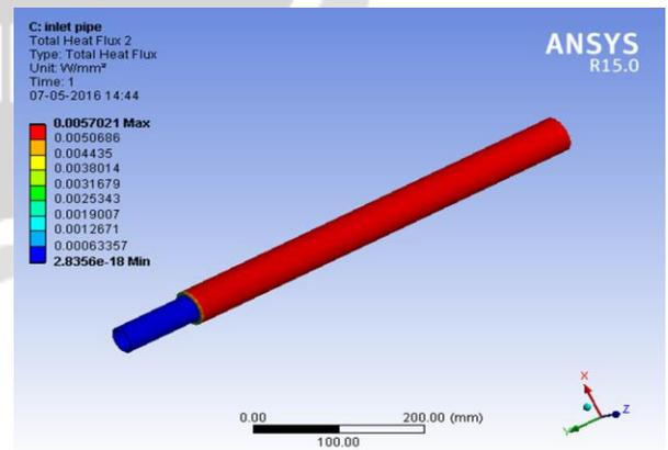
Fig. 21 Heat Flux Distribution in Liquid Helium Inlet Pipe
