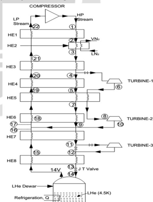
**Fig.1.** Process Flow Diagram of Indigenous Liquid Helium Plant (Courtesy: IPR)
