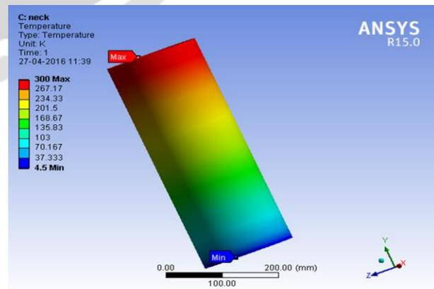
Fig. 18 Temperature Distribution in Neck
