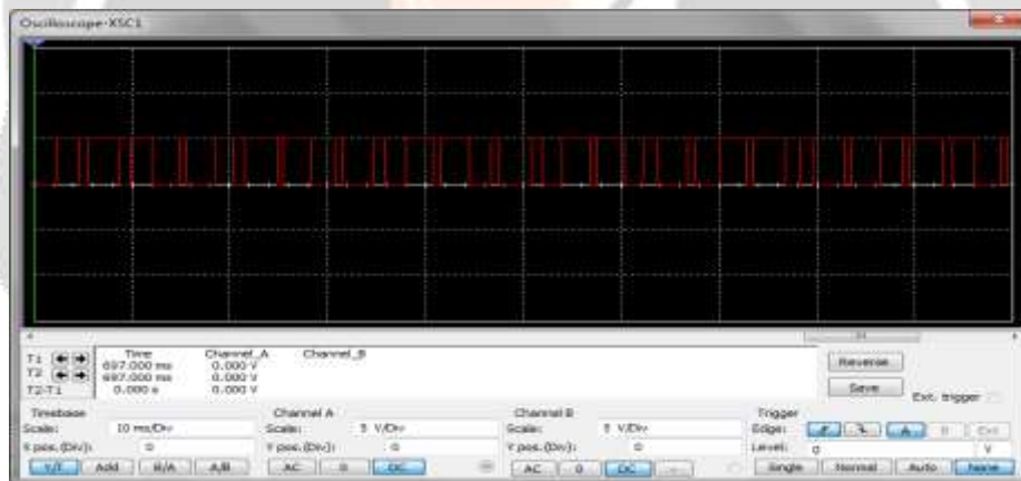
Fig. 6: Waveform of Analog to PWM generation.
