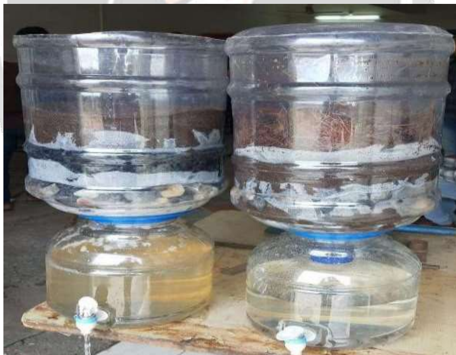
Fig.2 Experimental set up of Slow sand filters
